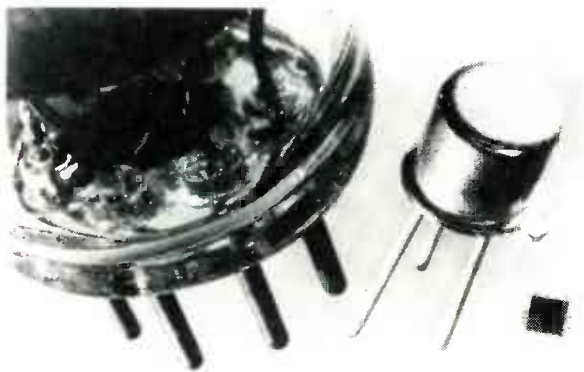
30 YEARS OF ELECTRONICS HISTORY IS represented in this photo: from left to right, a vacuum tube, a transistor, and an early integrated circuit.
