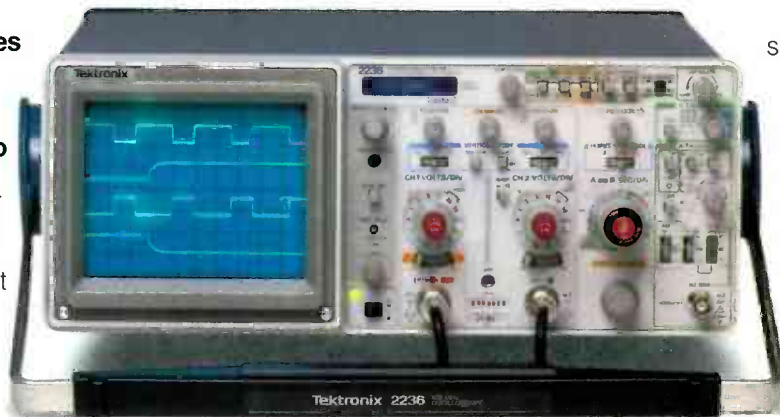
Gated frequency measurement. B sweep triggering during the intensified portion of the A sweep. Intensified portion frequency is measured with the counter/timer/DMM.
