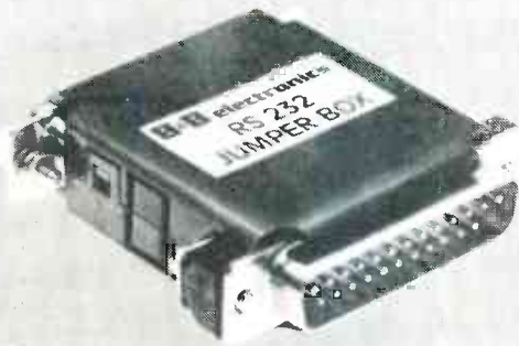
FIG. 10—This “D” connector shell is handy for wiring up RS-232 interface adapters. See the text for more information.
